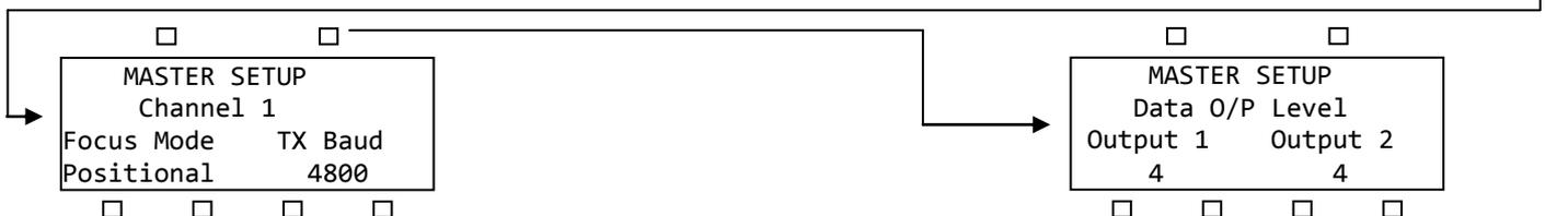
Focus mode should be set to 'Positional' for virtually all lens types. 'Rate' mode is only required for very specific lens types such as the Canon VCL-719BXS.
